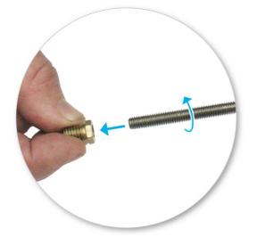
Select four grubscrews and assemble them into the adaptor using 3 mm (1/8") Hex Key.
