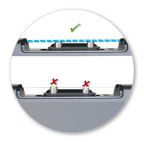
Place washer at base of spacer to adjust height if required.
