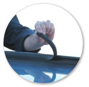
• Locate and remove rubber seal from inside edge of roof rail on vehicle.
